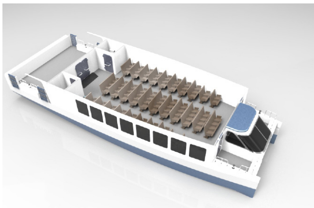
The ferry's 100-seat passenger deck was designed with "as little open area as possible", to dissuade overcrowding
